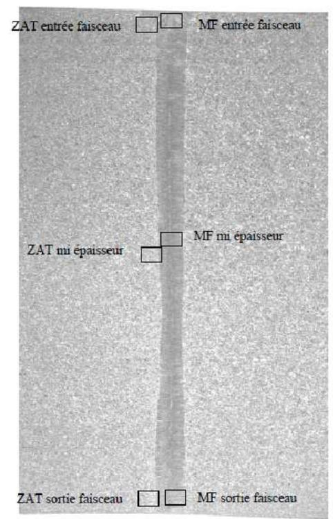
**Electron beam weld**
